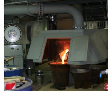
Melting furnace for NF metals
