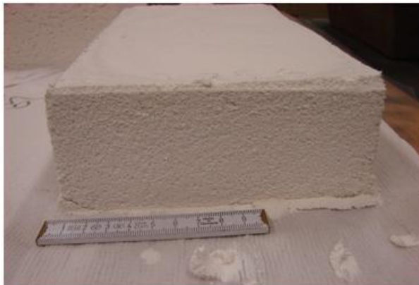
CA 6 sample after casting
