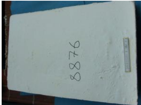
CA 6 block 600x400x100 mm after firing at 1625°C
